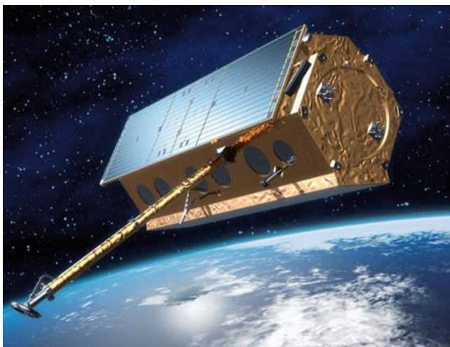
Fig. 13.7 Artist view of the TerraSAR-X satellite. Note the solar panel ( upper left ), the boom ( lower left ) with the X-band downlink antenna, and the X-band radar antenna ( lower right )
